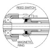
The magnetic field of the ring fixed on the nut activates the reed contact of the switch locked on the protective tube with a clamp.
