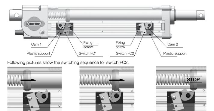
Standard switches have silver-plated contacts, max. current 12 A with resistive load - 6 A with inductive load. Switches with gold-plated contacts, very low contact resistance for low working voltage (if connected to PLC or PC), max. current 0.1 A, available on request.
